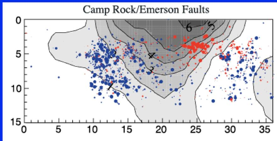
Stress drop (blue high, red low) along one fault segment from 1992 Landers – variable along fault – inversely correlated with high slip (*Shearer et al., 2006*)
